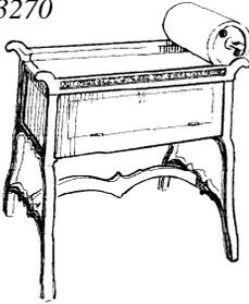
Roller proof press made by Chandler & Price, Cleveland, Ohio, about 1900. Height 41, width 24, length 4, cylinder diameter 9.
