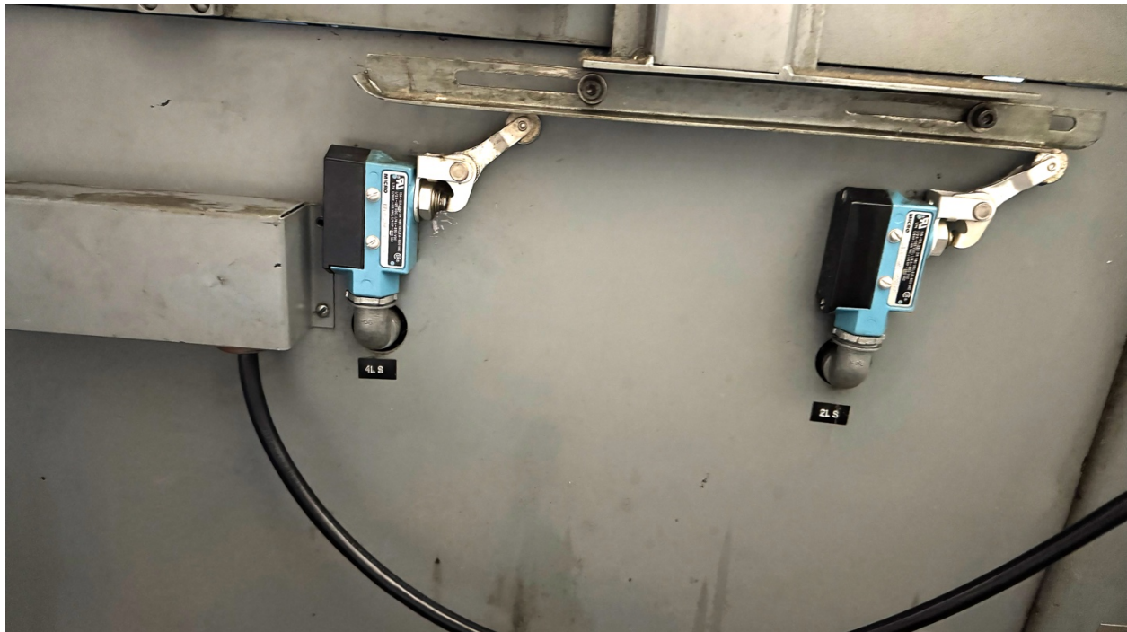
Figure 47 :The 4LS (left) and 2LS (right) BZE6-2RQ2 limit switches at the feed board end of the press. These micro switches with roller arm actuators are replacements from the original micro switches on the press.
